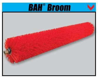
The TYMCO Broom Assist Head (BAH) standard rotary broom is constructed of virgin polypropylene bristles, each having a diameter of .078 and forming a 12 inch diameter around a schedule 40 pipe. Unlike "will-fit" brooms, every TYMCO BAH broom comes with a new bronze hub helping deliver excellent performance every time. Will-fit" brooms either do not come with a new hub or may come with a weaker plastic hub.
